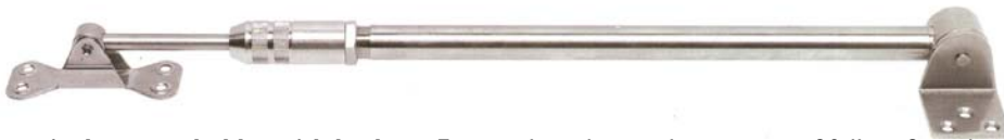
#32.500 Telescopic door stay holder with brake For medium heavy doors, up to 80 lbs. Stainless steel. Adjustable tension by turning nut. Stroke: 225 mm. Stainless steel. Overall length: Center to Center Brackets: 575 / 350 mm.
